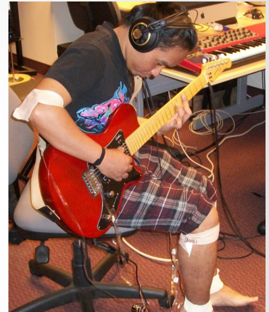
A whole-body tactile display for novice guitar players [Giordano, 2011]
