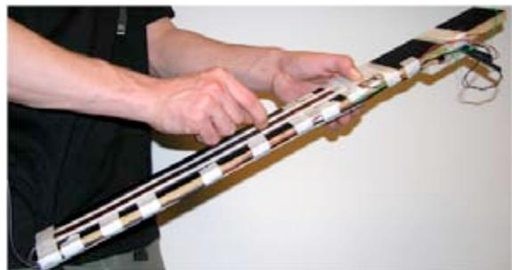
Fig. 13. The *CheapStick*, a low-cost USB controller using alternative touch sensors.
