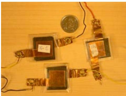
Fig. 12. Three homemade paper FSRs using metal contacts. Each FSR has different electrical characteristics dependent on the number of paper sheets stacked.
