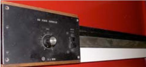
Fig. 1. The *Moog Ribbon*, a touch position sensor, part of the Moog Modular Synthesizer.
