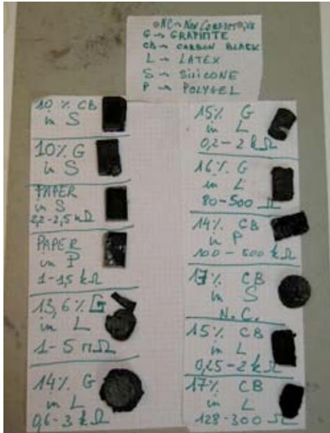
Fig. 5. Various samples made of composite materials.
