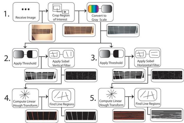
**Figure 9.** Strings and Frets detection using the linear Hough transform algorithm
