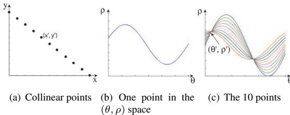
**Figure 6.** The normal parametrization of the line: (a) Ten collinear points; (b)  $\rho$  as a function of  $\theta$ , applying equation 3 for fixed parameter  $x$  and  $y$ ; (c) Intersection of the concurrent curves representing the ten points in a.
