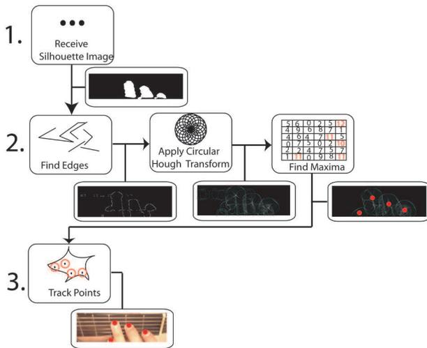
**Figure 8.** Fingertips detection using the circular Hough transform algorithm
