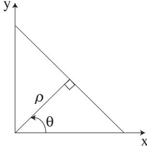
**Figure 5.** Normal parametrization of a line given by equation 3 where  $\theta$  and  $\rho$  are fixed parameters
