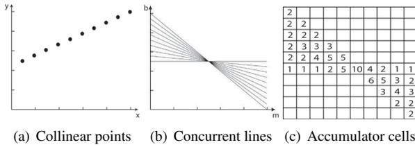
**Figure 4.** Example of 10 collinear points: (a) Collinear points; (b) Concurrent lines; (c) Accumulator cells.
