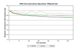
Figure 3: Resistance drift with time, 1000 g load for 1200s.
