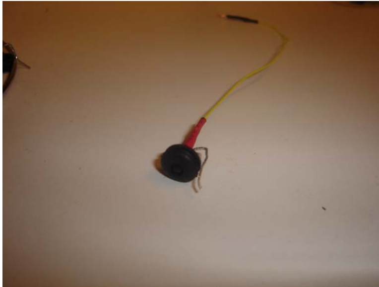
Figure 3-9: Infrared detector with rubber grommet for mounting on track
