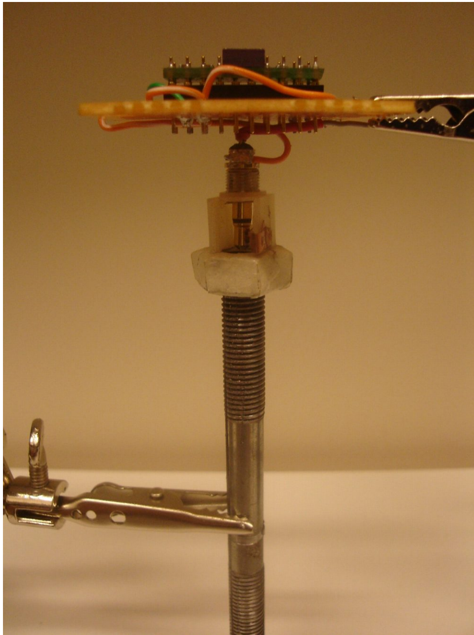
Figure 3-7: The axle, gyroscope sensor contact, and gyroscope sensors
