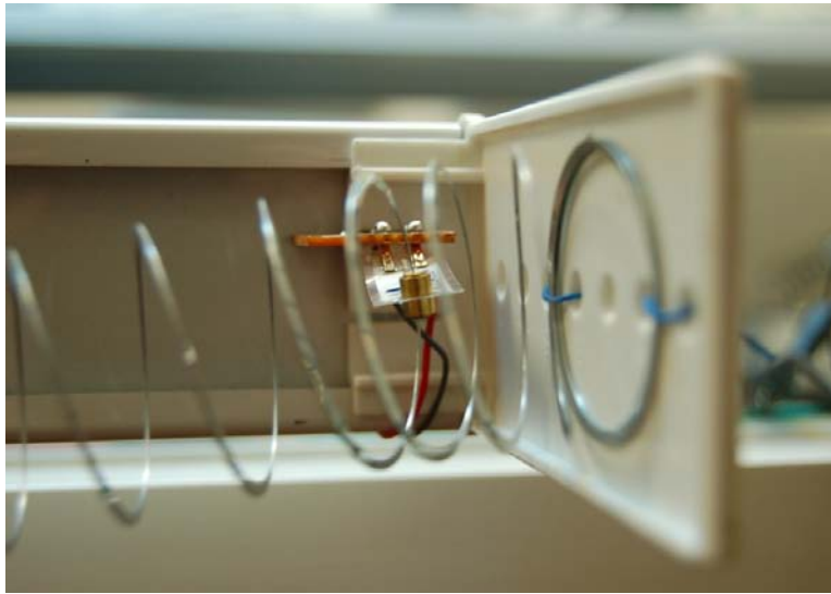
Figure 4-7: The piezo-film element is coupled to one end of the spring to measure percussion on the spring.
