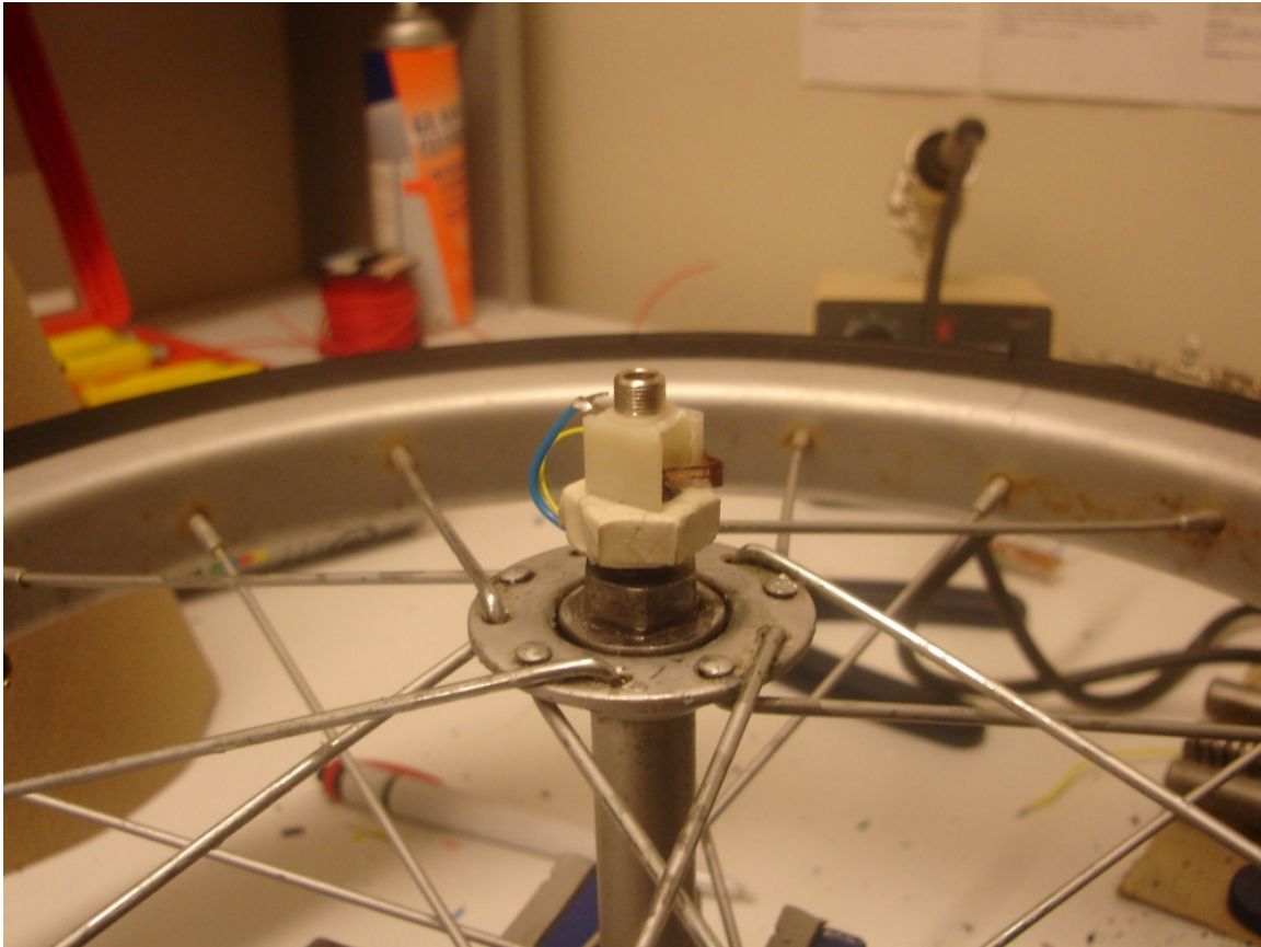
Figure 3–8: Gyroscope Sensor Contact (Second Version) mounted on the axle
