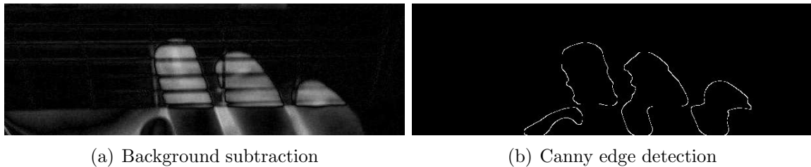
Figure 6.9 Segmentation steps of the fingering algorithm: (a) Result of background subtraction of the grayscale image of figure 6.8(b) from the grayscale image of figure 6.8(a) (b) Canny edges detection applied on (a)
