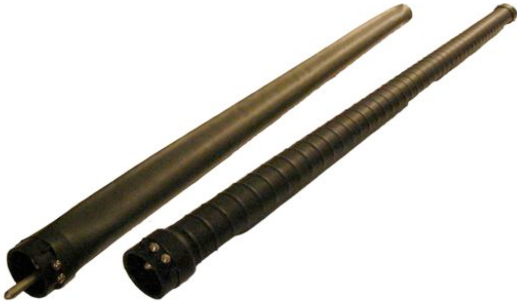
Fig. 3.2 The first T-Stick covered, shown before and after shrinking the tubing with a hot air gun.
