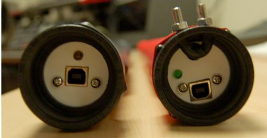
Fig. 3.3 A view of the endcaps of two T-Stick prototypes, showing the USB ports and status LEDs. Note the hole and fastener for the spike on the right.
