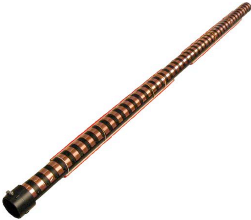
Fig. 3.5 The first T-Stick prototype before being covered, showing the strips of copper tape used as key electrodes for touch sensing.
