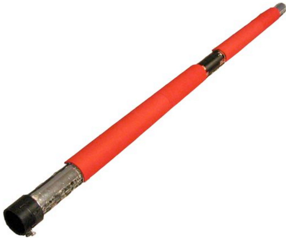
Fig. 3.8 A view of the back of the first T-Stick, showing the closed-cell foam padding used to cover the pressure sensors.
