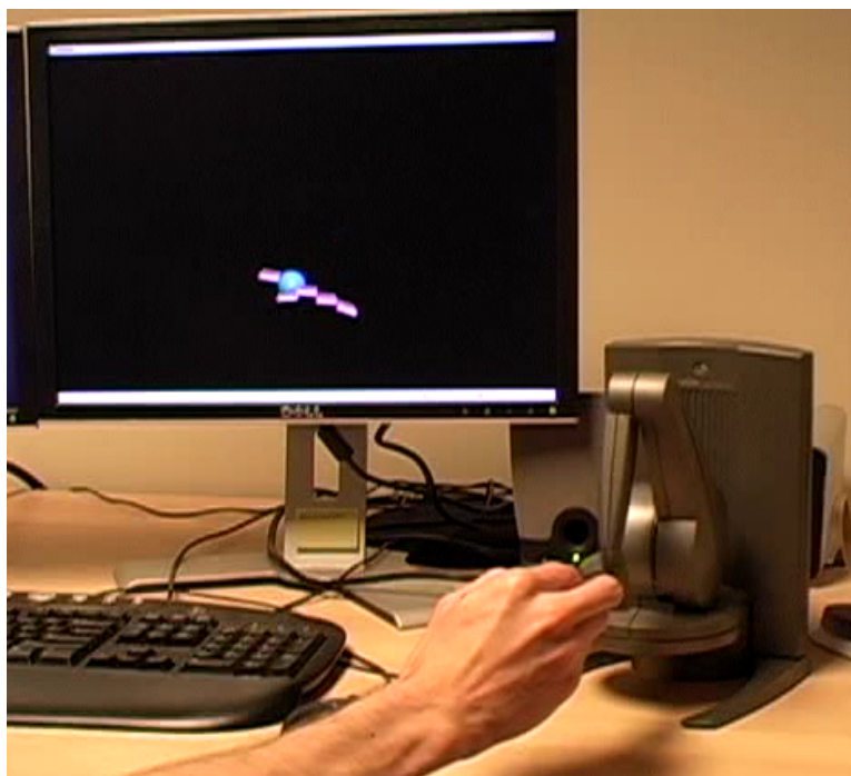
Fig. 4.9 A photograph of a user interacting with Chained FM using a Sens-Able Phantom Desktop. The prism objects are connected by springs. The movement of these objects produces parametric changes in an FM synthesis algorithm.
