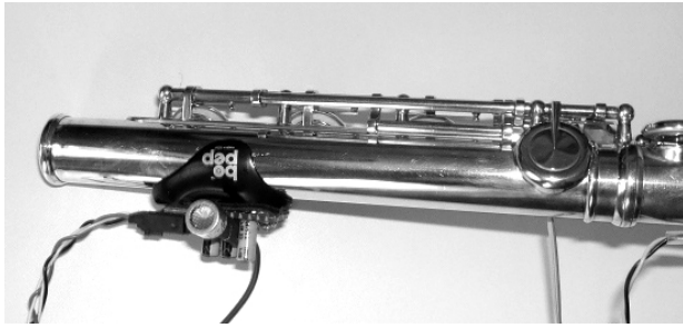
Figure 2. The accelerometer and ultra-sound transducer mounted on a Bo-Pep for the new hyper-flute.
