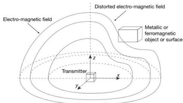
**Fig. 2.6** Magnetic tracker accuracy degradation, adapted from (Burdea and Coiffet 2003)
