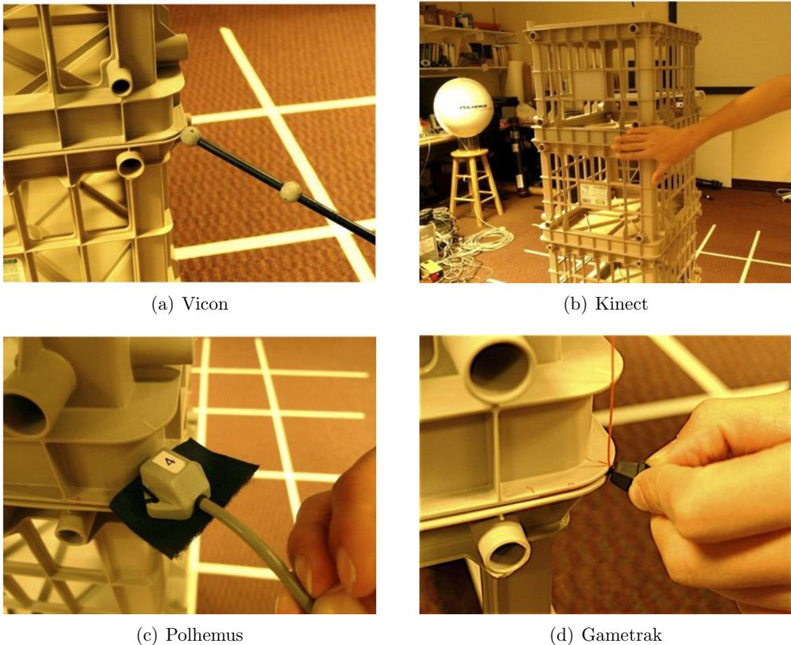
**Fig. 4.5** Measurement of the same point in space with the four tracking systems
