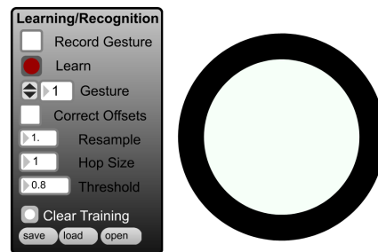
Figure 2: Graphical user interface (GUI) for the gesture recognition system (left). A GUI widget provides visual feedback to the guitarist upon successful gesture recognition (right).
