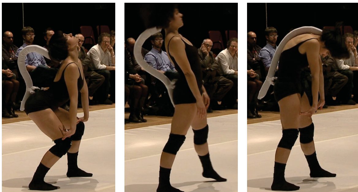
Fig. 5.4 A foam spine prototype with embedded sensing of orientation and shape in use during a public post-workshop presentation. Dancer: Sophie Bréton.
