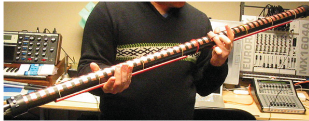
Fig. 2.2 An image of the first T-Stick prototype before being covered by the shrink wrap, adapted with permission from [15].
