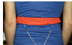
Figure 3. A test subject wearing our tactile display.
