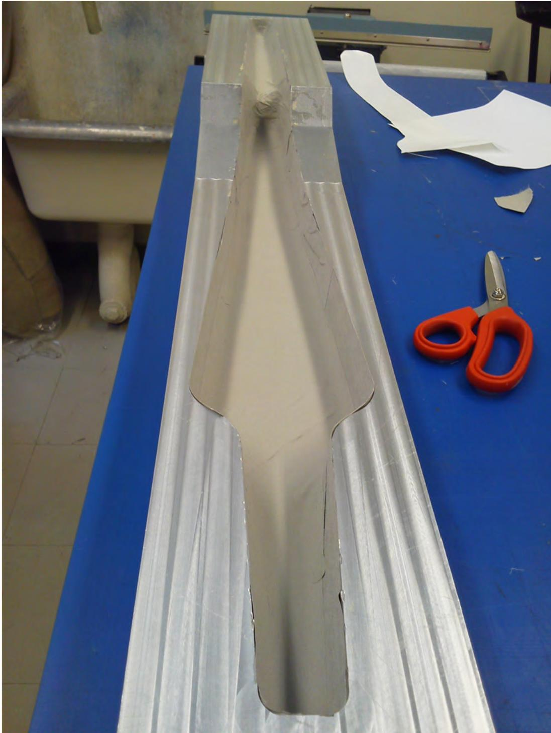
**Figure 6.5:** Aluminium cello body mould during initial stages of layup.
