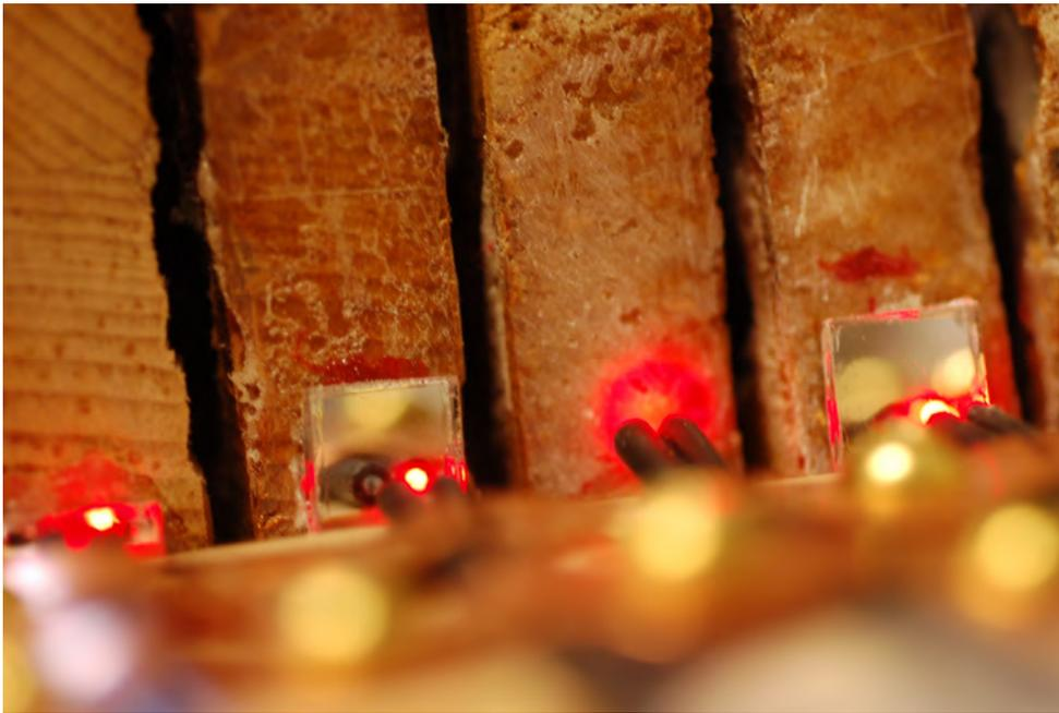
**Figure 5.2:** First piano prototype with mirrors on backs of keys aligned with emitting and receiving fibres [113].
