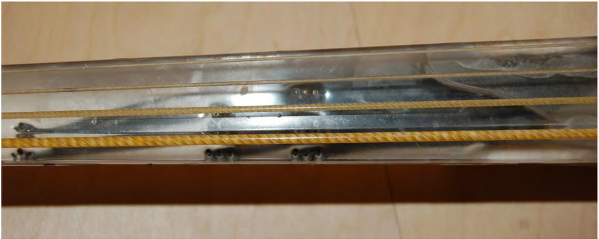
**Figure 6.18:** Transparent urethane fingerboard cast with POF mounted on cello body.
