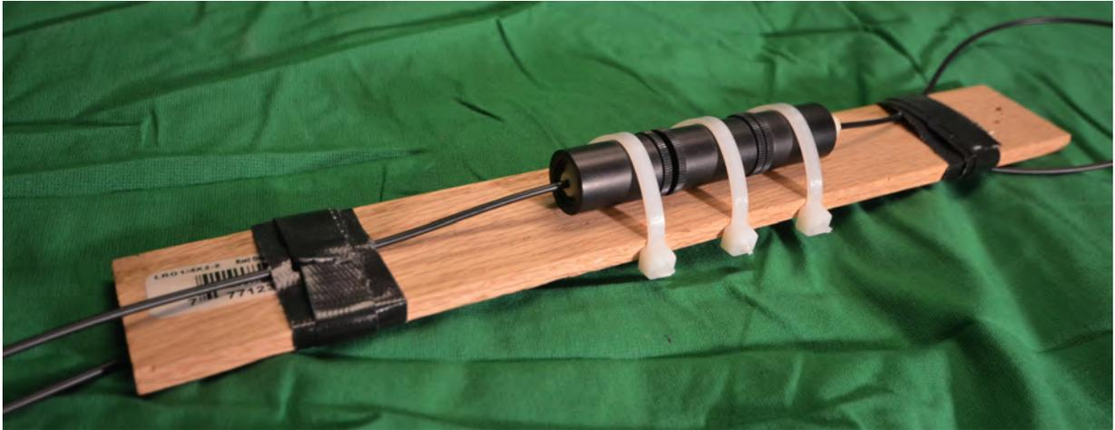
Figure 6.35: Prototype Faraday rotator in aluminium lens tube.
