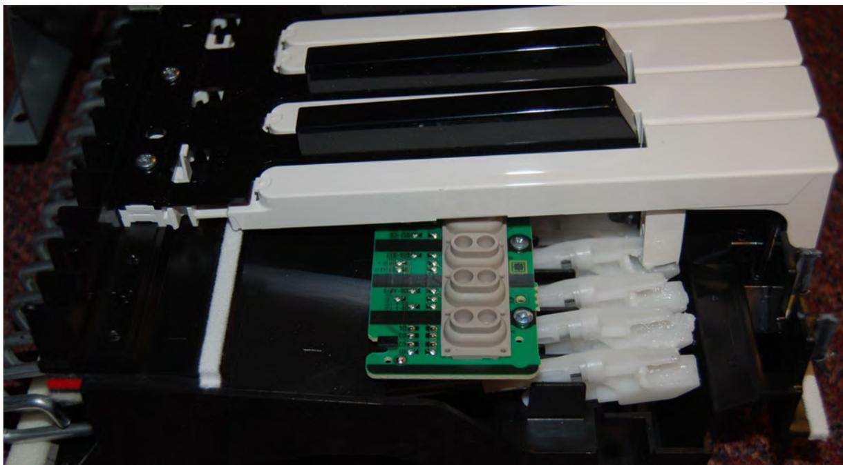
**Figure 5.5:** Yamaha electronic piano internals, with ferromagnetic counter-weight beams, screws, and electronic circuit board.
