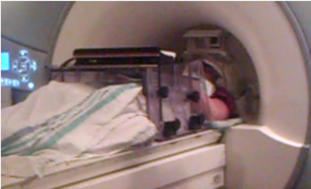
**Figure 5.19:** MRI-compatible keyboard in MRI scanner.
