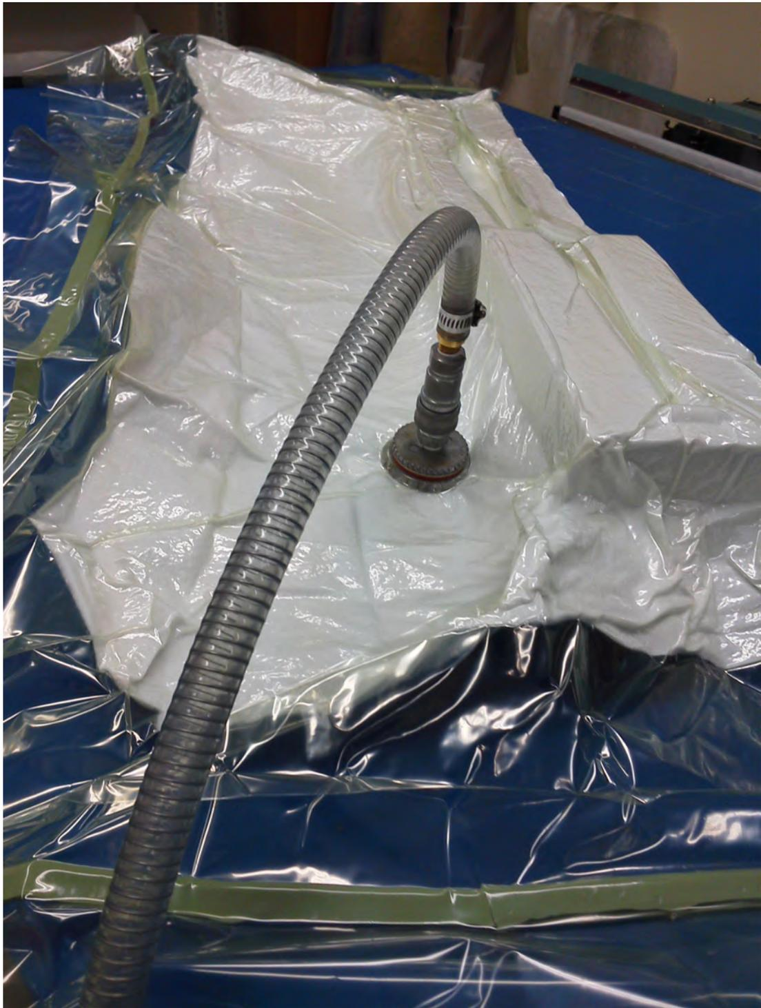
**Figure 6.10:** Composite cello in vacuum bag and conformal protective envelope, ready for heat-curing.
