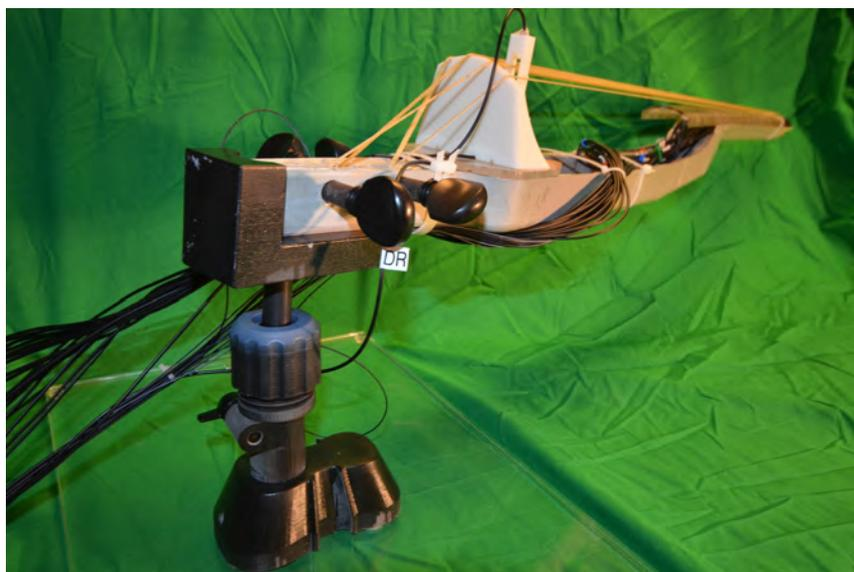
Figure 6.42: Cello supported in MRI-compatible fixture.
