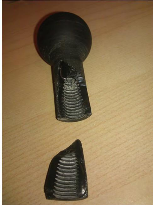
Figure 6.41: Material failure of 3D-printed ball joint.
