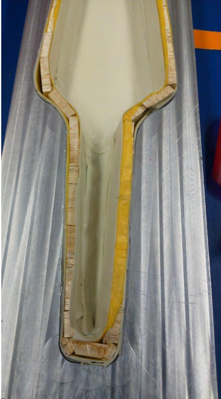
**Figure 6.9:** Composite cello layup with second set of fiberglass prepreg.
