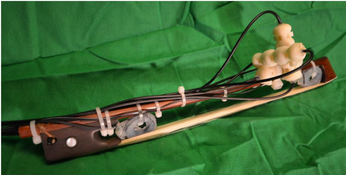
**Figure 6.30:** MRI-compatible cello bow with bow force sensors mounted at tip and frog, and 3D magnetic field sensor.
