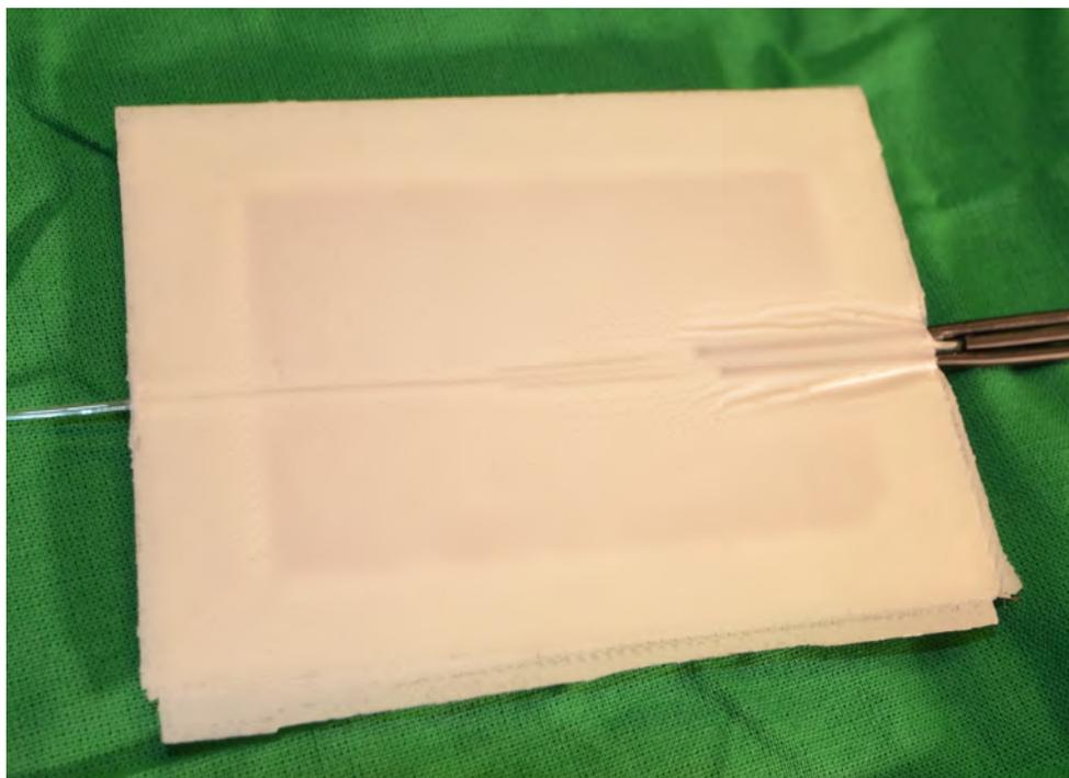
**Figure 6.12:** Fingerboard test fixtures with embedded optical fibres: composite fiberglass touch sensor).
