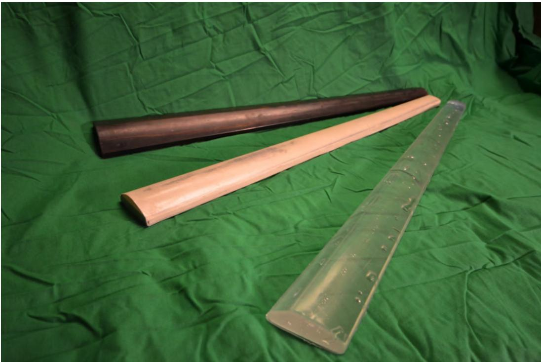
**Figure 6.15:** Wooden (top), fiberglass (middle), and cast transparent urethane (bottom) cello fingerboards.
