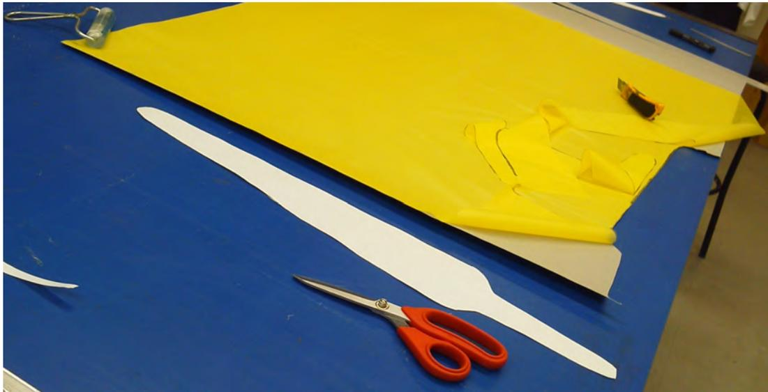
**Figure 6.6:** Paper template preparation for cello body.
