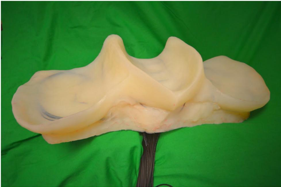
Figure 4.8: The Ballagumi, silicone interface with embedded fibre optic sensors.
