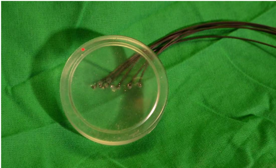
**Figure 6.16:** Transparent urethane test piece cast with 0.5 mm POF.
