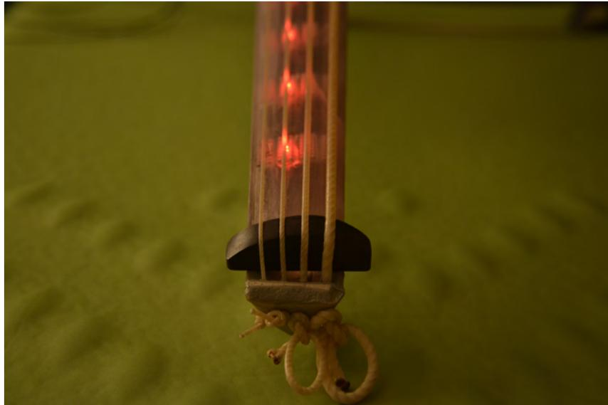
**Figure 6.21:** Transparent 3D-printed fingerboard mounted on cello body with gut strings.
