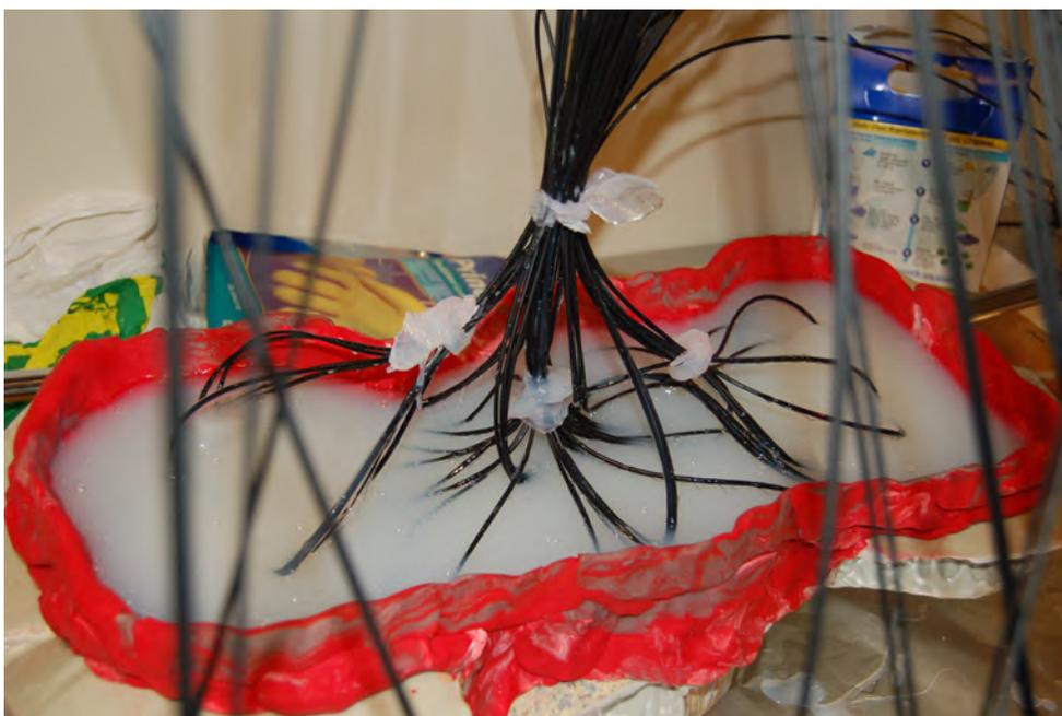
**Figure 4.7:** The Ballagumi with sensors potted before final silicone pour.
