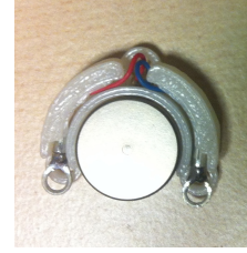
Figure 7: 3D printed housing for connecting the motors to the garments.
