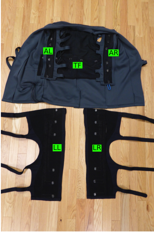
Figure 5: The final version of the garment. The actuators are clearly visible on the two leg modules and on the jacket (sleeves and waist). The green labels show the name of the modules as they are referred to in Sec. 4.2.
