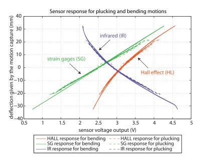
**Fig. 4.7** Sensor response for bending and plucking motions: deflection given by the reference measuring system, in mm, versus the sensor output, in Volts. The use of the apparatus limits the measurement range to a monotonic range, free of saturation.
