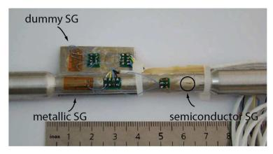
**Fig. 3.6** Metallic and semiconductor strain gages. The reference ruler has 1 mm resolution. Photo by Edison da Rosa. Reproduced with permission.
