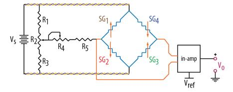
**Fig. 3.9** Conditioning circuit: full bridge with zero nulling adjustment. inamp circuit is shown in Figure 2.9. Arrows illustrate sign of strain when force is applied downward in the beam showed in Figure 3.10.
