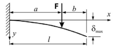
**Fig. 4.3** A concentrated force **F** is applied at a given point. The distance between the load and the clamped edge is a and the distance between the load and the free edge is b. The deflection at the free edge  $\delta_{max}$  depends on the beam material, beam geometry, force magnitude **F**, distance between load and clamped edge a and length of the beam b.
