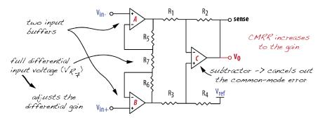
Fig. 2.9 Instrumentation amplifier [43].
