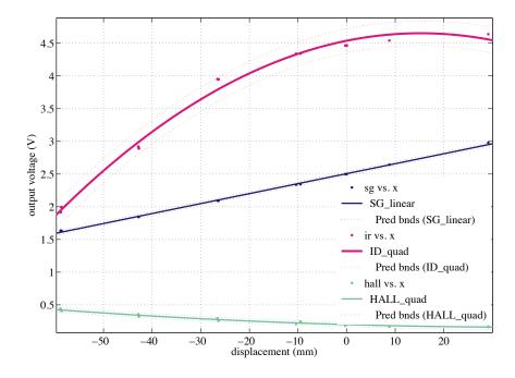
Fig. 3.12 Regression curves for each sensor
