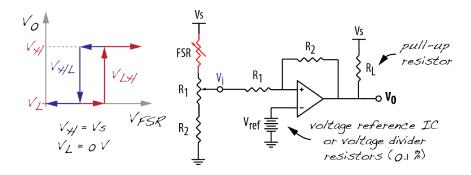
Fig. 2.10 Comparator with hysteresis based on IC manufacturer [102].
