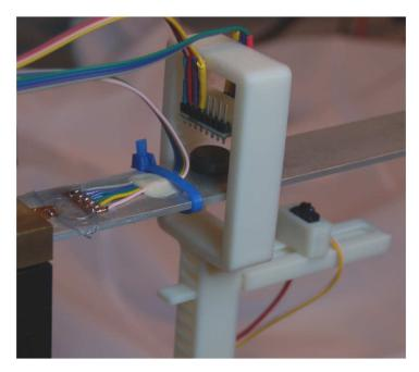
Fig. A.3 Detail of sensor placement for *The Rulers*. The following adjustments are available: independent discrete vertical position for IR and Hall effect sensors, and continuous longitudinal position for the IR sensor in relation to the Hall sensor longitudinal position. Apparatus design is a collaboration with Anthony Piciacchia. Photo by Vanessa Yaremchuk. Reproduced with permission.
