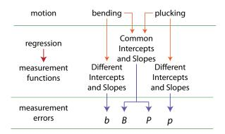
**Fig. 4.8** Sensor evaluation method. b, B, p, P are the suffix letters to be assigned to the sensor name. Letter b/B represents bending samples; letter p/P represents plucking samples. Lower case letters represent Different Slopes and Intercepts regression results, whereas upper case letters represent Common Slopes and Intercepts regression results.
