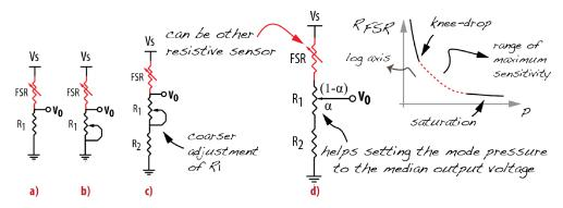
Fig. 2.7 Voltage divider topologies. (a) simplest solution; (b) output offset adjustment; (c) safety improvement; (d) safety and finer adjustment. Solution a is suggested by one FSR manufacturer, solutions b and c are often found on DIY designs, and solution d is proposed by us.
