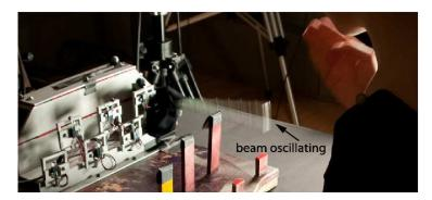
**Fig. 4.4** Performer executing **plucking:** free beam oscillation originated by an initial driven deflection. Photo by Guillaume Pelletier. Reproduced with permission.
