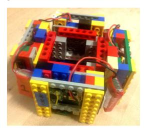
**Fig. A.5** Building for MARG sensors calibration. The design has a space in the center for the hand. This allows the operator to perform random motions in all directions. The perpendicularity of the sensor placement allows verification of heading angle. Collaboration with MIT Media Lab Responsive Environments Group, Eric Berkson, and Tom Kepple.
