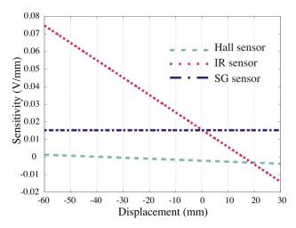
Fig. 3.14 Strain Gage, IR and Hall effect sensor sensitivities across the measurement range
