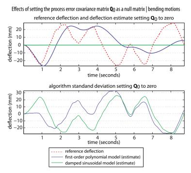
**Fig. 4.14** Effects of setting the process error covariance matrix as a null matrix, for **bending** motions. The top graph displays the deflection given by the reference measuring system, the deflection estimate given by a first-order polynomial filter, and by a damped sinusoidal filter (which does not estimate any deflection). The bottom graph compares the algorithm standard deviation for both model settings.
