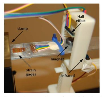
Fig. A.2 Apparatus for sensor placement for *The Rulers*: based on LEGO bricks and 3D printing. LEGO bricks are used to add flexibility (discrete adjustment of vertical position) and to reduce cost. Rail fitting allows continuous adjustment of longitudinal position for the Hall sensor. Apparatus design is a collaboration with Anthony Piciacchia. Photo by Vanessa Yaremchuk. Reproduced with permission.
