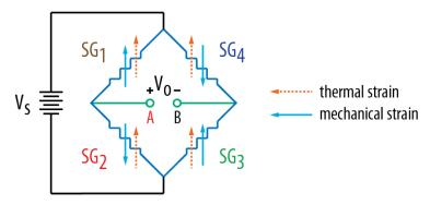
Fig. 3.8 Example of Wheatstone bridge for being strain measurement with temperature compensation.
