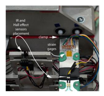
Fig. 3.2 Sensors placement and clamp.
