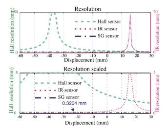
**Fig. 3.15** Strain Gage, IR and Hall measurements resolution across the range. The bottom graph is a zoomed version of the top one, highlighting resolutions lower than 5 mm.
