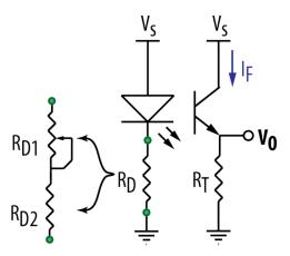
Fig. 3.3 QRD1113 polarizing circuit
