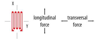
Fig. 3.7 Bonded metallic strain gage grid: design maximizes sensitivity to longitudinal strain—measurement of interest—and minimizes sensitivity to transversal strain. Transversal sensitivity is the sensitivity to strain in the sensor's transversal dimension.
